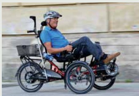
Scorpion Plus: when you pedal the motor assists up to 15mph. Armrests, high seat, similar trikes fold up.
